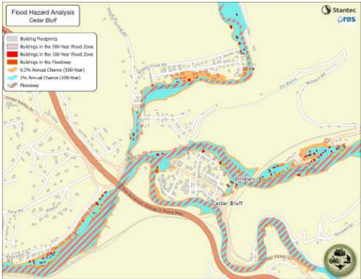
Figure 633: Flood Hazard Analysis – Cedar Bluff Area
