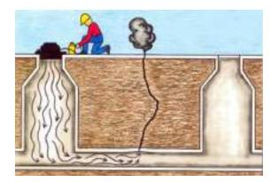
Figure 721: Smoke testing for I/I<sup>5</sup>
