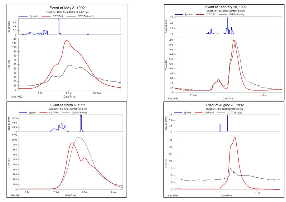
Figure 4-9: Modeled vs Observed hydrographs for four events at Falling Creek Gage
