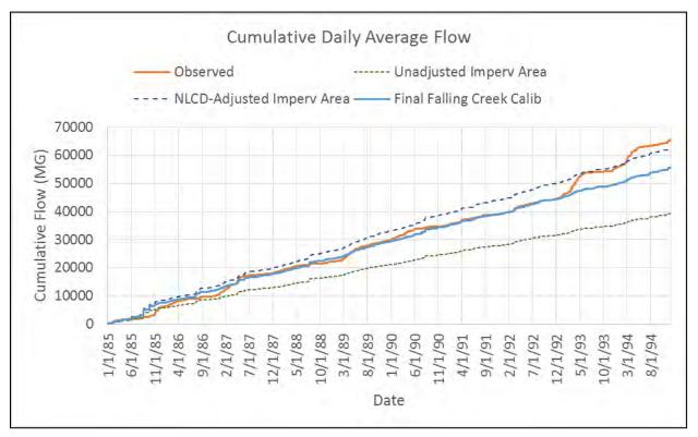
Figure 4-10: Model calibration results (impervious area)
