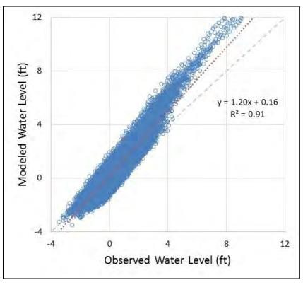
Figure 4-15: One-to-one Comparison of Modeled and Observed Water Levels at downstream USGS gage without calibration of water levels at the boundary
