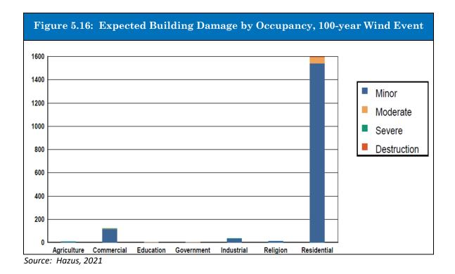
Hazus was also used to model summary building damage estimates based on percentage of damage (by damage state) for the 100-year return period (**Figure 5.16**). These data can be useful when used in conjunction with Table 5.16 above because building wind damage can range from minor, easily repairable damage to gutters or roof features, to destruction of roofs and buildings from fallen trees, or structural failure.
