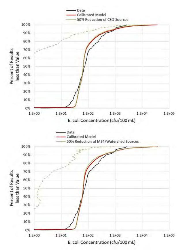
Figure 4-22: Sensitivity of Model Results to 50% Reduction of Wet Weather Sources
