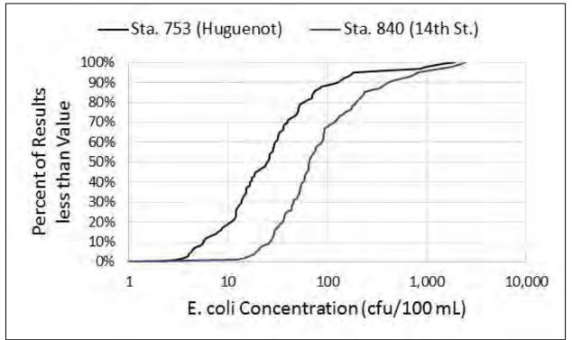
Figure 4-2 compares cumulative frequency distributions (CFDs) at the upstream station and a station near downtown. Median (50<sup>th</sup> percentile) *E.coli* concentrations increase from 25 to 66 CFU/100 mL, indicating a significant persistent source of *E.coli* to the river between these locations.
