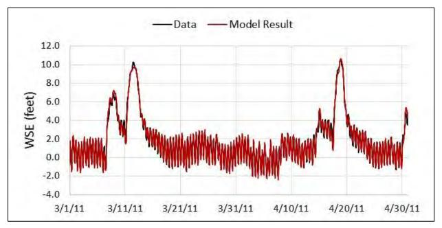
Figure 4-13: Time Series Comparison of Modeled and Observed Water Levels at downstream USGS gage
