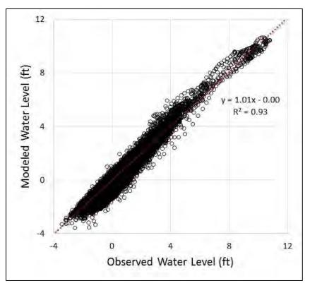
Figure 4-14: One-to-one Comparison of Modeled and Observed Water Levels at downstream USGS gage
