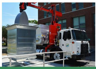
Figure 7. Submerged refuse container in Kissimmee, Florida (Zero Waste Design Guidelines)
