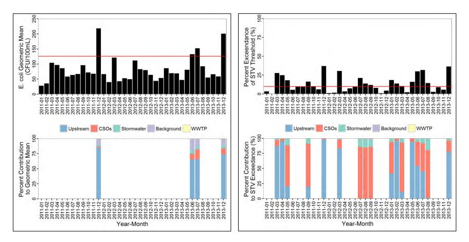
Figure 3.2. E.coli Monthly Geometric Mean and STV Standard Model Results for Current Conditions
