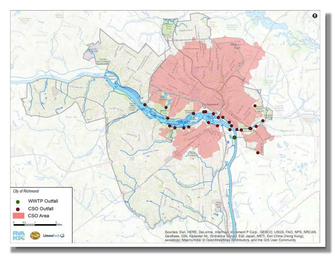
Figure 3.1. Combined sewer overflow area within the City of Richmond and location of CSOs
