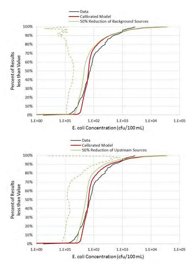
Figure 4-21: Sensitivity of Model Results to 50% Reduction of Persistent Sources
