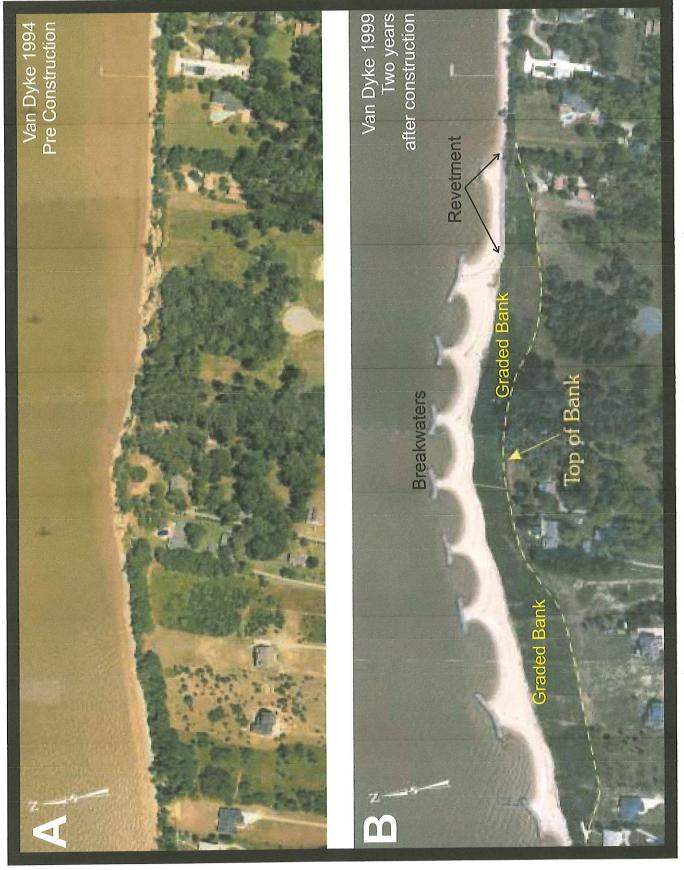
Figure 10. Non-rectified aerial photography of Van Dyke A) before installation and B) after installation.
