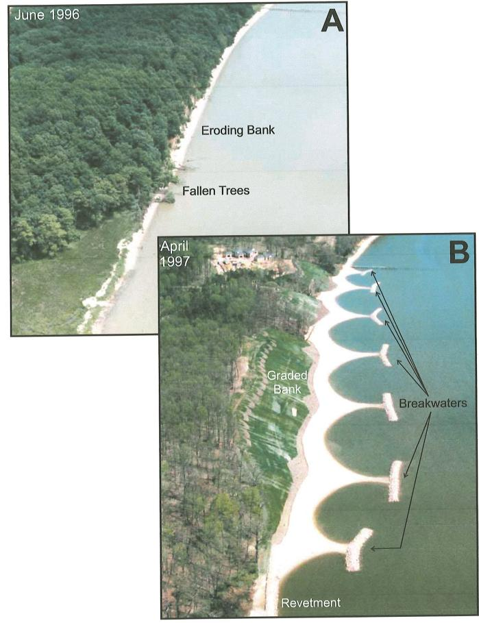
Figure 9. Photo of Kingsmill A) before installation and B) after installation.
