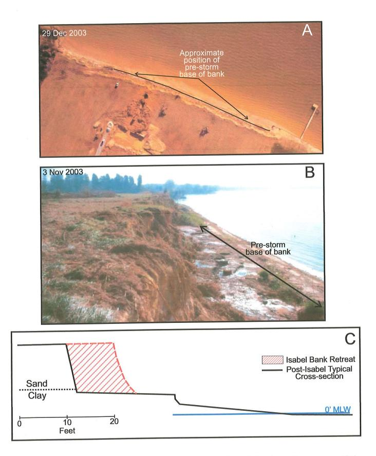
Figure 33. Impacts to the unprotected shore at Lenhart due to Hurricane Isabel shown A) on a non-rectified aerial photo, B) ground photo, and C) on a typical post-storm cross-section.
