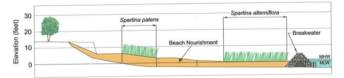
Figure 6. Breakwater system on Patuxent River in Calvert County, Maryland and a typical breakwater cross-section.
