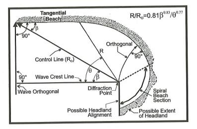
Figure 2. Parameters of the Static Equilibrium Bay (after Hsu et al., 1989).
