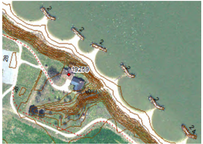
VIEW OF BREAKWATERS AND TOMBOLO FEATURES ALONG THE SHORE OF THE JAMES RIVER IN ISLE OF WIGHT COUNTY. BREAKWATERS ARE A PREFERRED METHOD OF SHORELINE STABILIZATION.
