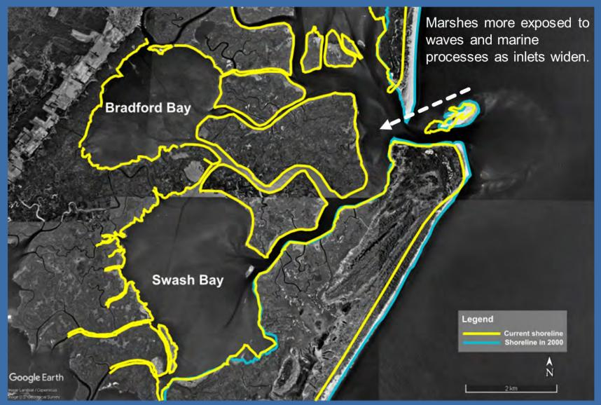
Wave impacts and water levels in the marshes are determined by the barrier island evolution, and the storage of sand in shoals.
