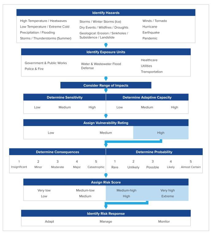
Figure 7: Sample Illustration of Vulnerability and Risk Assessment Process Flow
