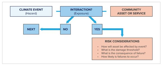
Figure 5: Decision Workflow for Assessing Exposure of Assets to Natural and Non-Natural Hazards
