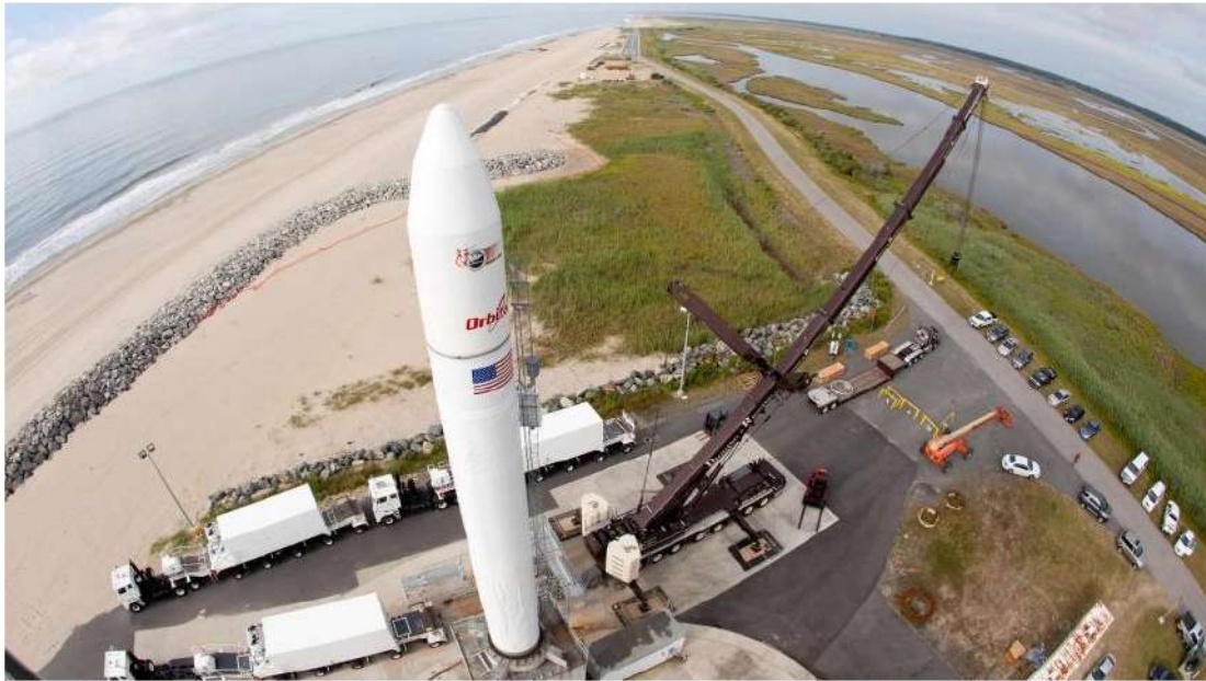
A wide-angle view of an inert Minotaur V launch vehicle is erected on the Mid-Atlantic Regional Spaceport's pad 0B at NASA's Wallops Flight Facility in Virginia during a pathfinder exercise for NASA's Lunar Atmosphere and Dust Environment Explorer (LADEE) Mission.
