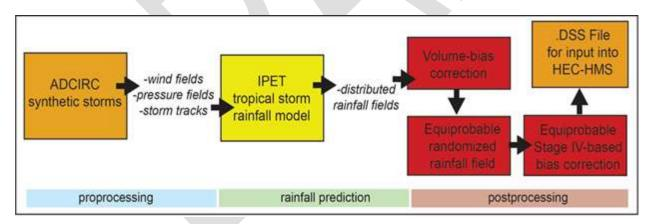
Figure 18: Workflow of the synthetic rainfall generation methodology, including a preprocess step that creates input parameters for the IPET parametric rainfall model and a postprocess step that improves the predictive ability of the IPET model for use in the study area.
