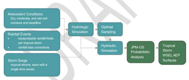
Figure 15: Workflow of synthetic storm boundary and initial conditions development, numerical simulations, and statistical analyses for tropical storms.
