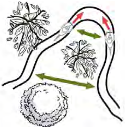
Green, horizontal arrows indicate adequate sight lines that allow riders to see oncoming traffic. Courtesy IMBA/Rich Edwards.
