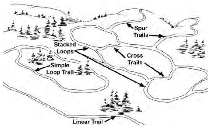
Linear, loop, spur, and cross trails. Courtesy of USDA Equestrian Design Guidebook.
