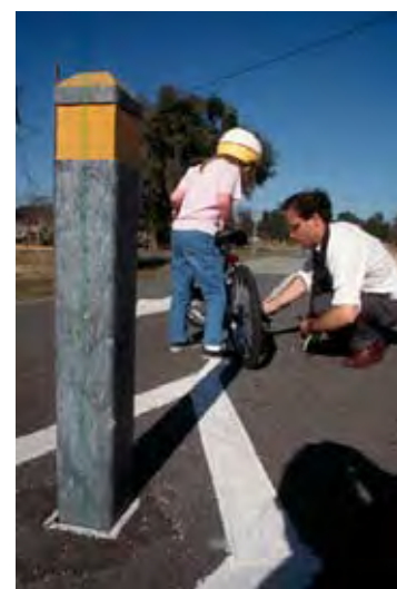
Left: Retractable metal bollards slide into a sleeve set in the ground when not in use. Courtesy of LPDA, Inc. Right: Removable bollards pull out of the ground completely. Courtesy of www.pedbikeimages.org /Dan Burden.
