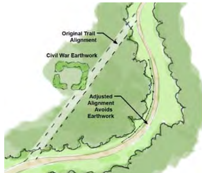
Adjusting trail alignment to avoid sensitive resources. Courtesy of LPDA, Inc.
