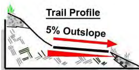
Outslope drainage on a trail. Courtesy IMBA/Rich Edwards.
