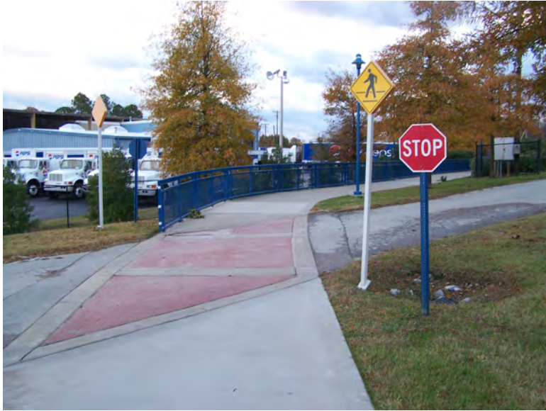
What is wrong with this photo? All crosswalks must be bordered with retroreflective white striping. Signs do not conform to MUTCD guidelines.
