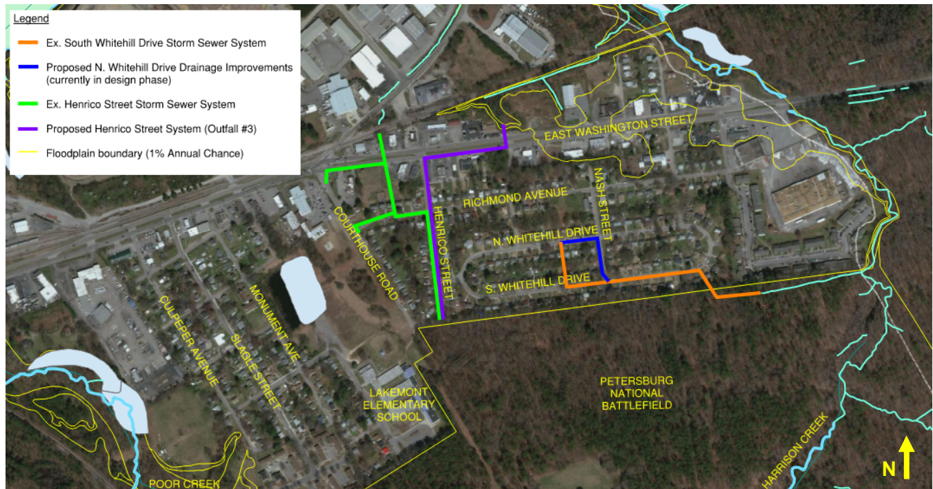
Figure 1. Storm Sewer Systems in the Whitehill neighborhood.
