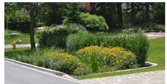
With dense vegetation, absorbent soils, and underground storage capacity, rain gardens help treat stormwater and prevent flooding of homes and streets. Photo courtesy of CNT/RainReady.
