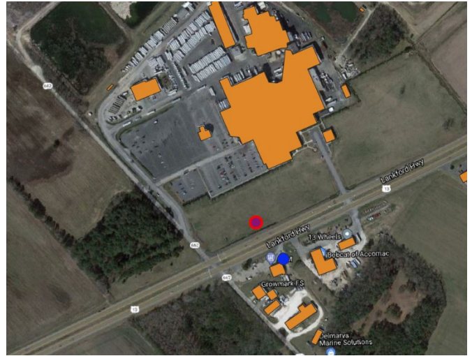
Figure 5: Example of challenge in aligning assets to building footprints. The selected point from the DHS Homeland Infrastructure Foundation-Level Data (HIFLD) represents a critical manufacturing facility, however only a manual assignment of the point to the facility's footprint, impossible to accomplish due to current time constraints, would have yielded an accurate location and thus a valid risk assessment.
